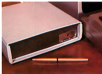
Photo 1: The Disk-80 mounted in its enclosure and attached to the TRS-80 Model I computer. The Disk-80 is about half the size of the Radio Shack TRS-80 Expansion Interface.
